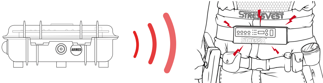
IED Adaptor sends signal to activate StressX™ belt
