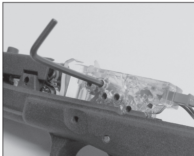
Figure 22: Adjust Trigger Break Location Cam with the 3mm hex wrench
