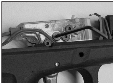
Figure 25: First Loosen Trigger Take-Up Spring Retaining Cam Cap Screw
