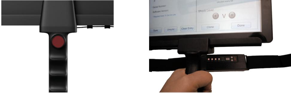
Face Ir sync window on Hand Grip Handle towards StressX™ Belt Ir sync window
