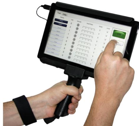
**NOTE:** The USB Cable connects the StressVest® Instructor Tablet to the software electronics housed in the pistol grip.
