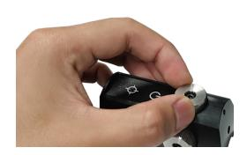
Once the laser is sighted, place the Sight Lock over the sighting dials to secure them in place (refer to the pictures below). Be careful not to move the sighting dials while placing the Sight Lock.
